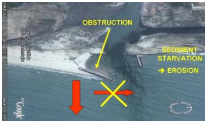
Figure 5: Illustration of shoreline impacts of breakwaters
